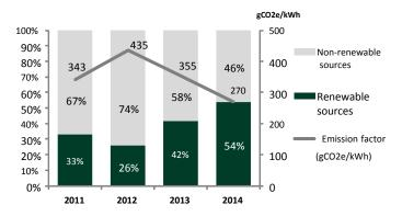
Fig. 7 – VdA's electricity source and carbon content in 2014.
